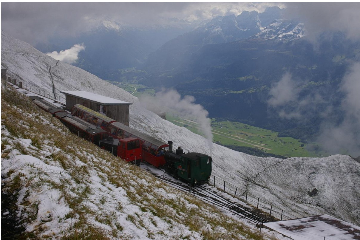
Plate 3: Series H 2/3 rack tank steam locomotive and its diesel competitor Hm 2/2 at Brienz Rothorn Station on September 5, 2007. Photographs: R. W. Serchinger.
