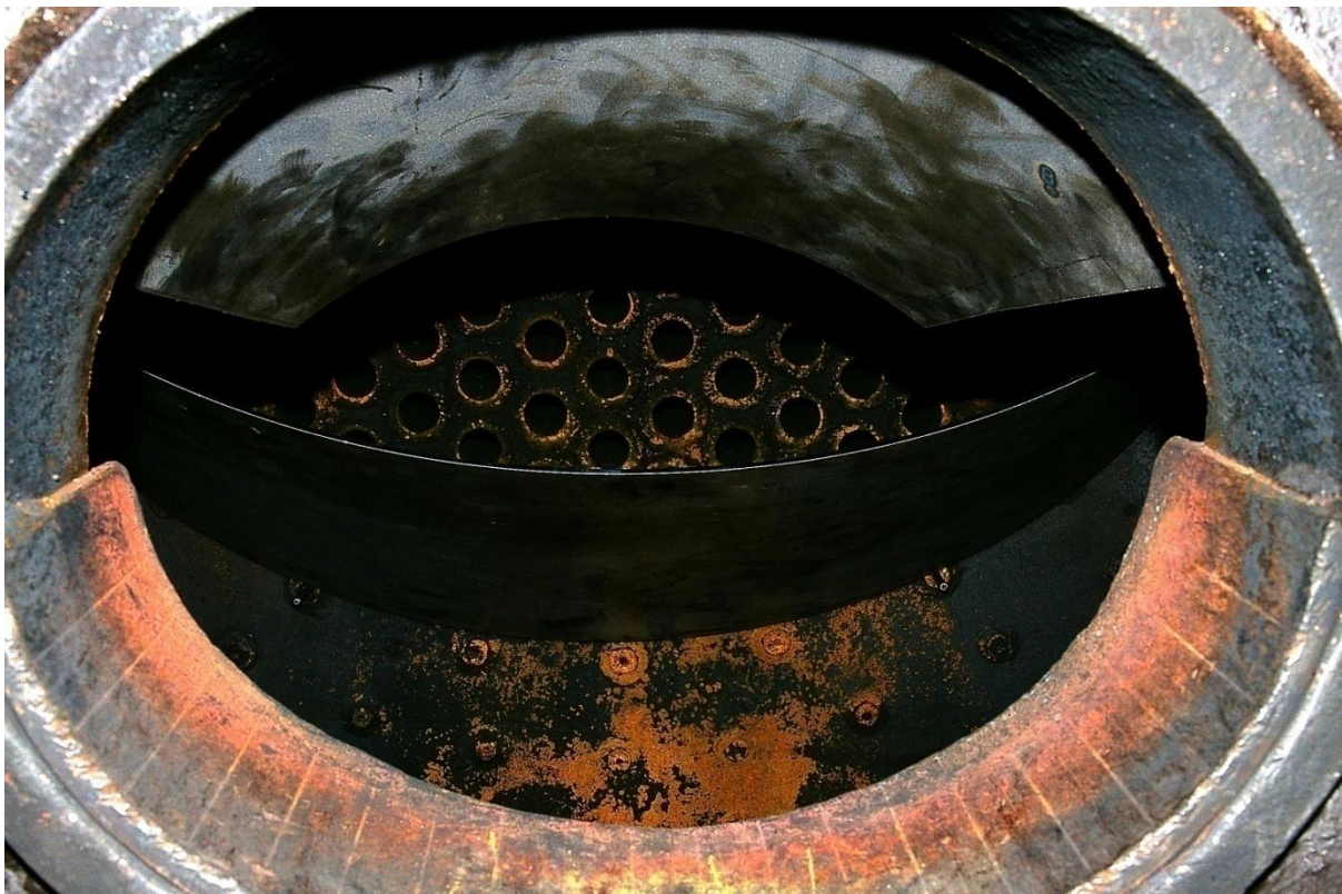
Plate 5: Inverted steel arch and deflector plate. Achenseebahn #1, experimental set-up with secondary air inlet in the firedoor, Jenbach, June 7, 2008. On a test run, this arrangement boosted fuel efficiency under full load by some 22 %! Photograph: R. W. Serchinger.
