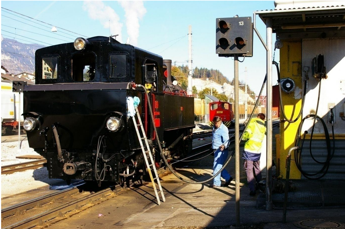
Plate 4: Zillertalbahn #5 is being refueled at the diesel locomotive fueling station, using standard diesel locomotive bayonet tank filler neck fittings. Jenbach, October 27, 2010. Photograph: R. W. Serchinger.
